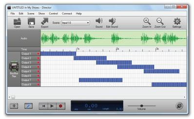
Once you create or open a show Director will automatically assign the digital outputs in your show to the Digital Output buttons. Any analog outputs will be assigned to sliders in the Analog Outputs section.
